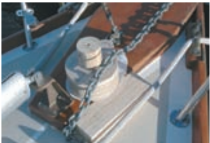
John used scale models to try out possible areas on the deck for the location of the windlass. The chain stretching aft pointed the way to the best location for the equipment.
