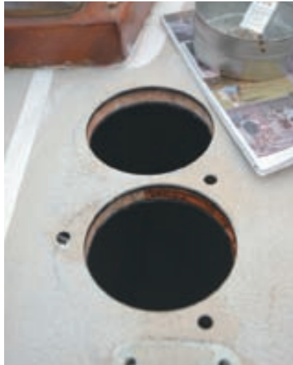
Once all the decisions have been made, it’s time to cut holes in the boat, above, and install the equipment, below. The aft hole is for the motor shaft. The forward hole is where the chain will pass through for storage below.
