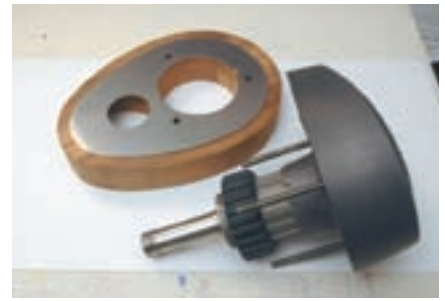
The raised teak base was constructed using the stainless-steel deck plate from the manufacturer as a pattern.
