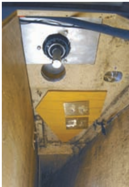
The windlass drive shaft (without the motor installed) protrudes through the stainless-steel backing plate. The chain drop hole is in the center. The previous hawser hole is the oval hole at the right. Notice the reinforcement plate for the windlass.
