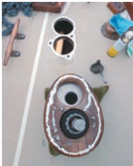
Once all the decisions have been made, it’s time to cut holes in the boat, above, and install the equipment, below. The aft hole is for the motor shaft. The forward hole is where the chain will pass through for storage below.
